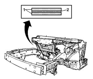
This information provides repair recommendations and general guidelines for steel classified as Laminated Steel. This type of steel is constructed by bonding 2 pieces of cold rolled steel (1) with a viscoelastic layer of adhesive (2).
